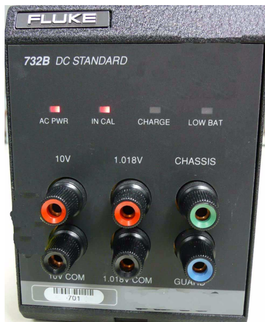
Fluke DC Standard 732B (ohne 1V)
